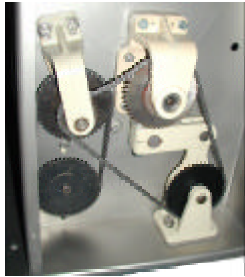
Flexible Drive Multiple Feedrates Are Available by Changing Sprocket Combinations
