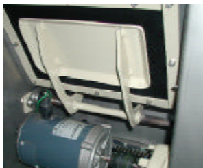
Low Density Material Conditioning Pulsating Hopper Agitation Insures Reliable Feed for Hygroscopic and Packing Chemicals
