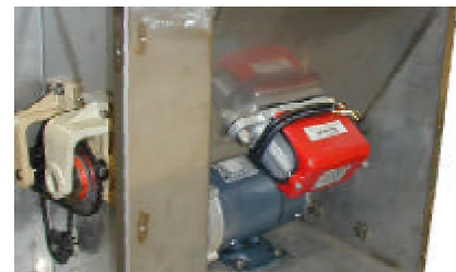
High Density Material Conditioning Vibrator Agitation Insures Reliable Feed for Heavy Granular Chemicals
