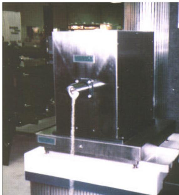
and discharge device are examples of components that contribute dead load to the weight the feeder must measure. The *live load* is the weight sensed from the material being fed.
