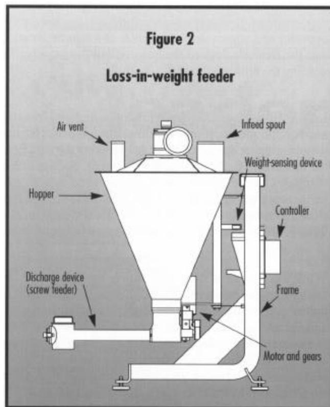
Assuming your LIW feeder's setpoint is in weight-per-minute units, calculate the feeder's accuracy for 30 1-minute samples using this formula:
