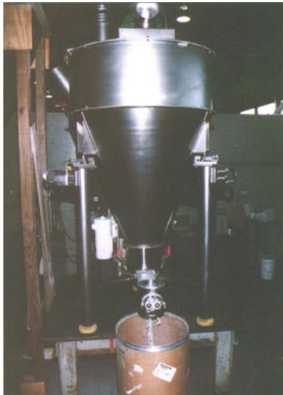
**b. Feeder mounted on platform scale**
